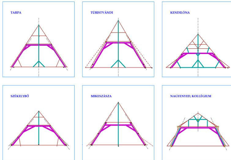
The features of shapes of roof structures with mixed and interim systems
