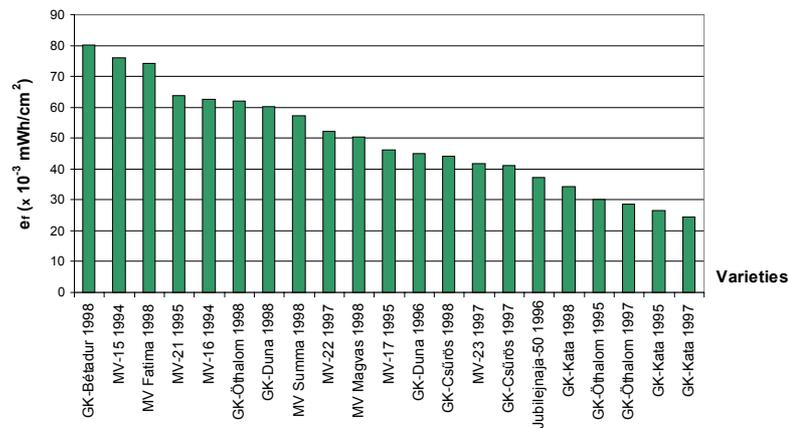
**Figure 2 Average grinding resistance ( $e_f$ ) of the investigated samples in descending order**
